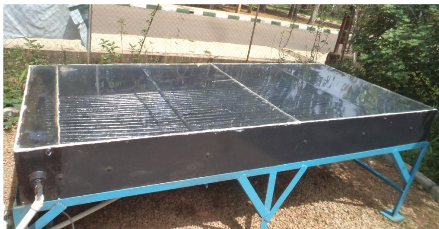
Figure 2b: Pictorial view of Solar Collector after Cover is placed on it
