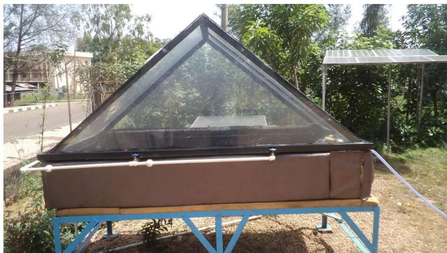
Figure 2b: Pictorial view of Solar Collector after Cover is placed on it
