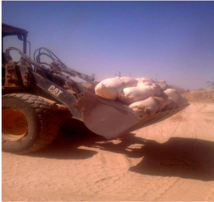
Figure 5: A Pay Loader Conveying Explosives
